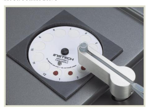
Optional dried blood spot disks, featuring Whatman FTA® DMPK-C paper, measure 6cm in diameter and hold 10 or 12 spots of 10 to 25µL. Blood samples may be spotted singly, in duplicate or in triplicate. Disks are easily replaced when more spots are to be collected.
