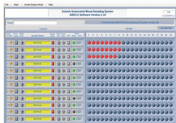
Control and monitor up to 12 samplers from a single PC. The main screen displays critical parameters for all units in real time, including which samples have been collected, unit status, cooler temperature and tee sensor readings.
