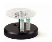
Removable carousel with numbered positions simplifies transport and identification of samples. Carousel is keyed so that the sampler will always place the first sample in position 1.
