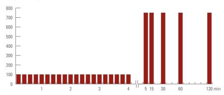
The software will first run the unit in a high-speed sampling mode, collecting as many as 20 samples of 20-100µL in 4-5 minutes, then autuomatically switch to a standard PK sampling mode, taking up to 20 samples over 24 hours or more.
