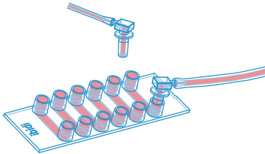
4. Open the clamped tubing and conduct your perfusion experiment.
